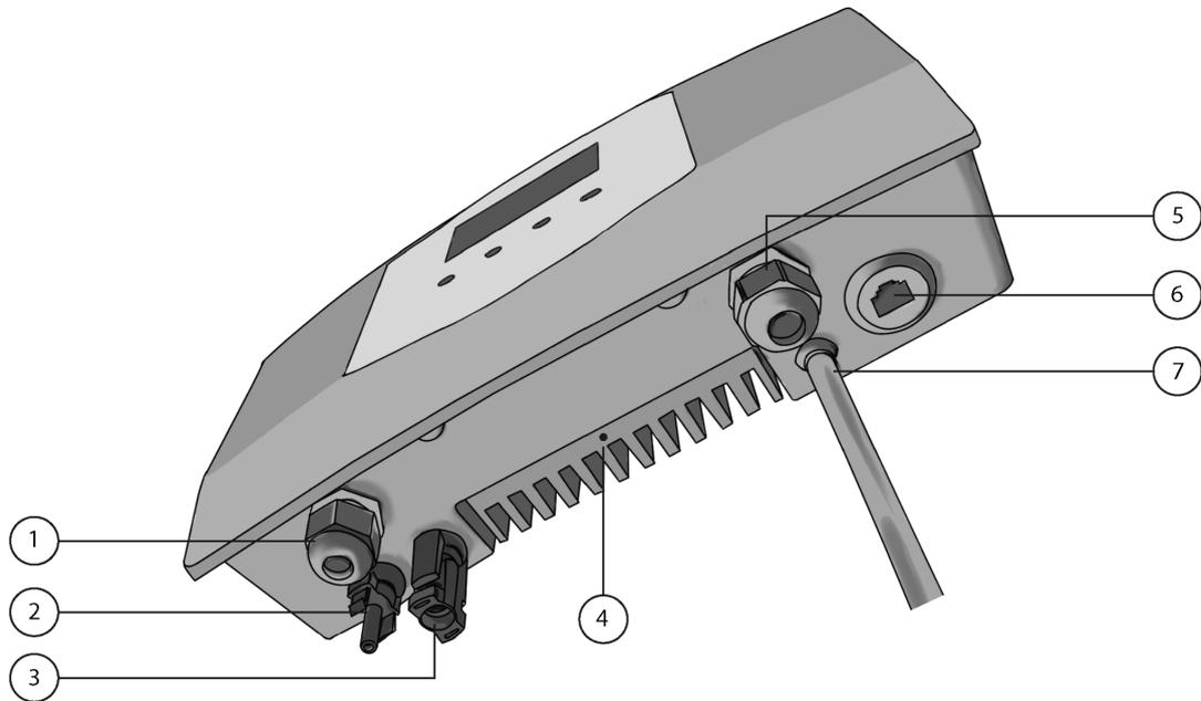
1. DC OUT - output for DC heating rods in the boiler
